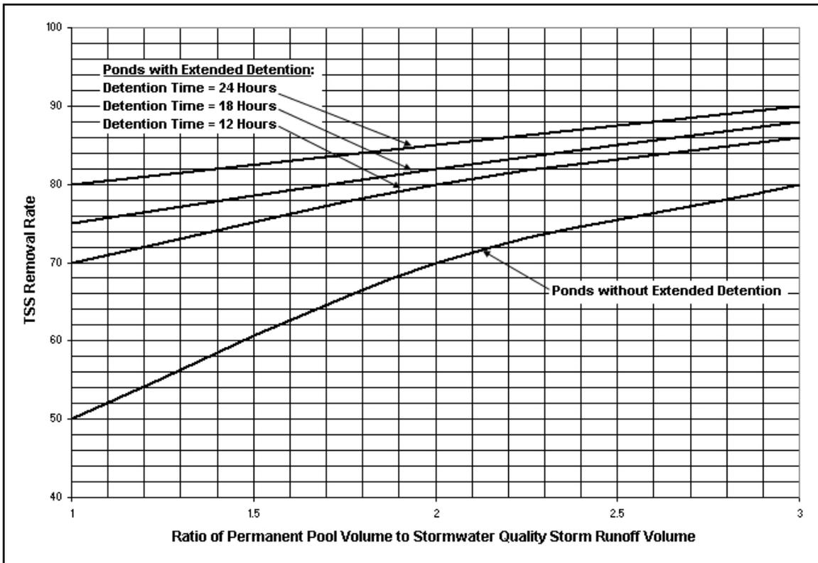
The following example illustrates how to use the chart to determine the TSS removal rate provided.
