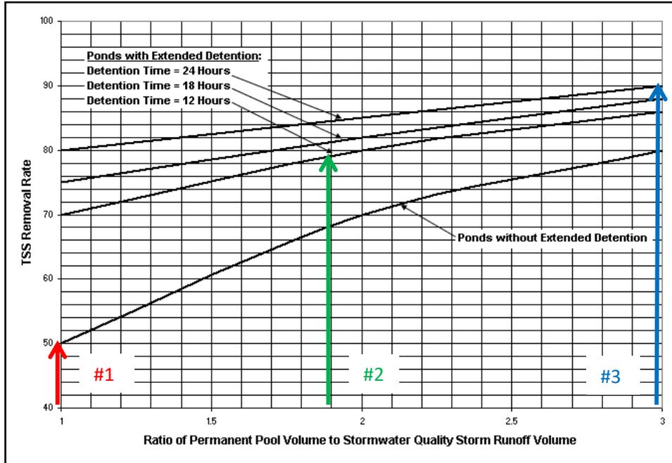
**Step 3:** For each of the designs, at the intersection of the vertical line from Step 2 with the respective curve, draw a horizontal line from right to left over to the y-axis to get the TSS removal rate.
