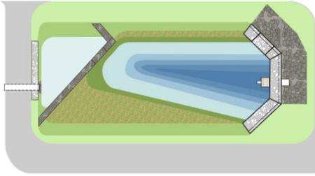
Wet ponds designed with a reuse component and a native vegetation perimeter are used to address the stormwater runoff quantity impacts of land development. This type of stormwater facility has an elevated outlet structure that creates a permanent pool where stormwater runoff is detained and attenuated. Wet ponds can be designed as multi-stage, multi-function systems; extended detention in the permanent pool provides pollutant treatment for runoff from the Water Quality Design Storm
